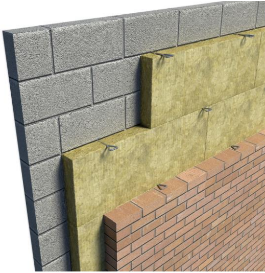
Figure 2 Wall tie positioning – Full fill application
