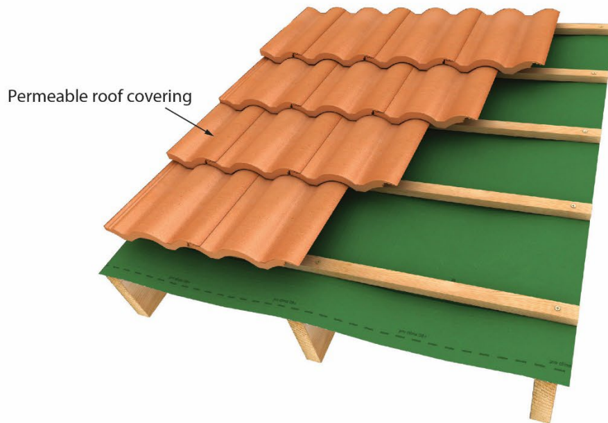
Figure 1: Cold Roof detail with permeable roof covering
